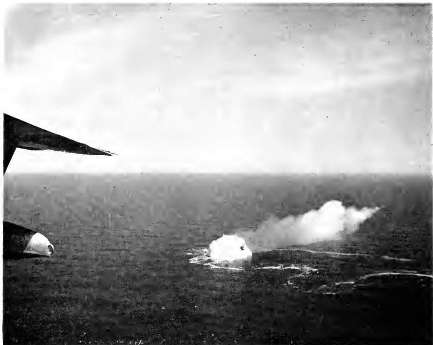
FIGURE 18.— Bomb drop on 10 June 1959. Center of impact of the cluster of 57 bomblets is the darkened crater on the right of the berg.
